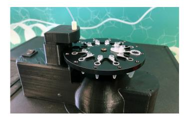
The Collector is controlled by the same software program that also coordinates the functionalities of the Photolysis, Radical Dosimeter, and integrated microfluidics systems. This unified software eliminates the need to monitor photolysis processing time to insure proper collection of labeled product without undue introduction of unlabeled sample.
