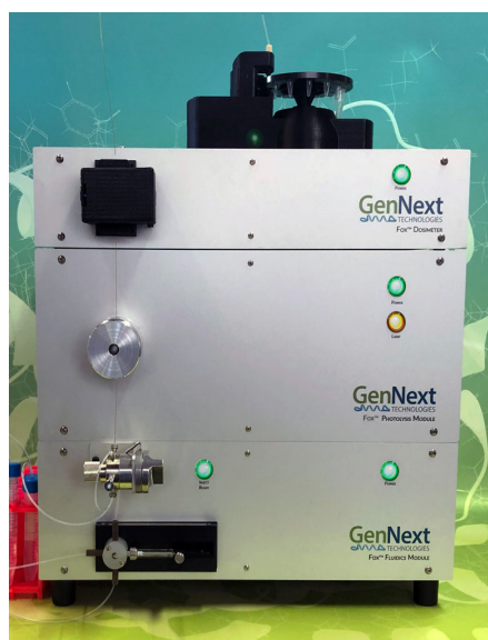
Fig 1: Flash Oxidation (Fox ® ) Protein Footprinting System
