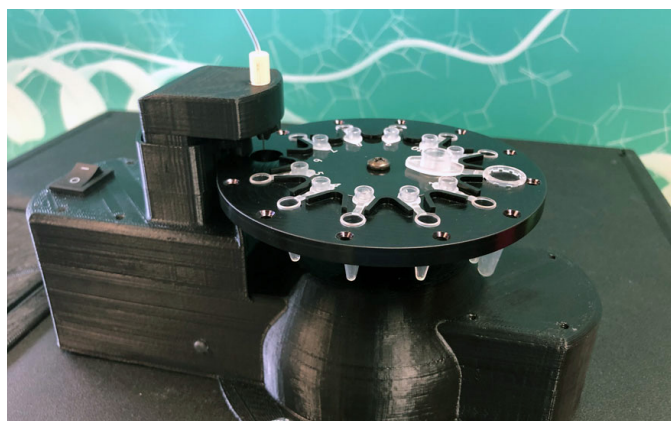
Fig 4: Fox ® Automated Product Collector
