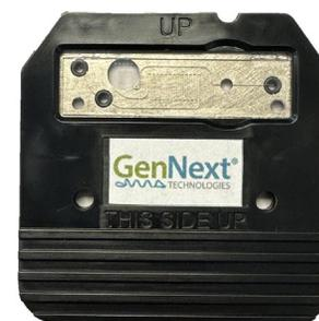
**Figure 1:** HRPF labeling is performed in an automated fashion using a 96-well plate in the AutoFox System. Sample delivery, reagent mixing, and flashing are performed through a microfluidic chip designed to maximize irradiated volume. Samples are quenched in an adjacent well prior to LC-MS/MS analysis.
