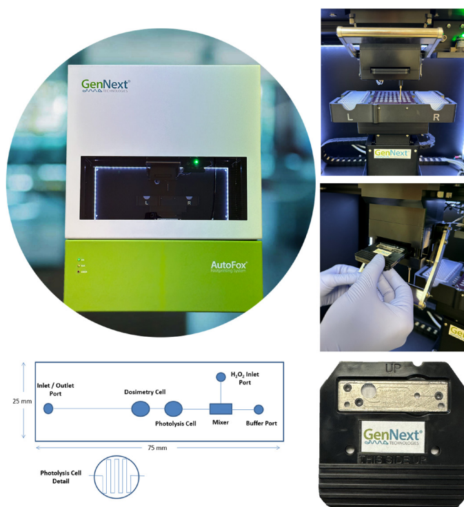
Figure 1: HRPF labeling is performed in an automated fashion using a 96-well plate in the AutoFox System. Sample delivery, reagent mixing, and flashing are performed through a microfluidic chip designed to maximize irradiated volume. Samples are quenched in an adjacent well prior to LC-MS/MS analysis.
