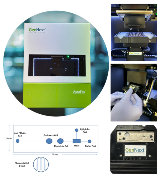
Figure 1: Automated & Reproducible Labeling. HRPF labeling is performed in an automated fashion using a 96-well plate in the AutoFox System. Sample delivery, reagent mixing, and flashing are performed through a microfluidic chip designed to maximize irradiated volume. Samples are quenched in an adjacent well prior to LC-MS/MS analysis.
